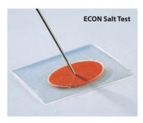
Eliminate rapid corrosion in lube oil, fuel or hydraulic systems by checking for the presence of salt.
