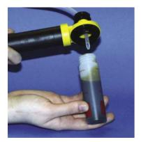
Effective predictive and preventative maintenance programs rely on scheduled oil sampling and analysis programs to provide an accurate indication of equipment and lubricant condition.
